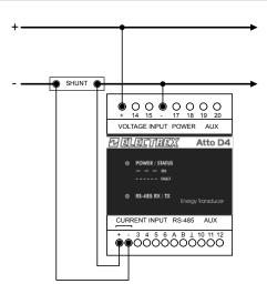
**POWER SUPPLY AND SERIAL LINE CONNECTION** The instrument is fitted with a separate power supply. The power supply terminals are numbered (17) and (18). Use cables with max cross-section of 2,5 mm<sup>2</sup> if stranded, 4
