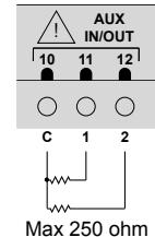
For loads with higher impedance of 250 ohms it is necessary to include in series an external power supply.
