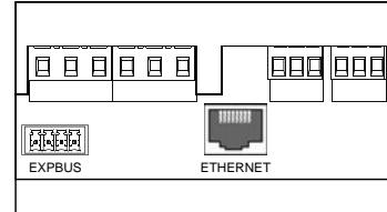
The instrument is equipped with a Ethernet Lan 10/100 Auto-MDI/MDIX port. For the connection can be used a data cable straight or crossover.
