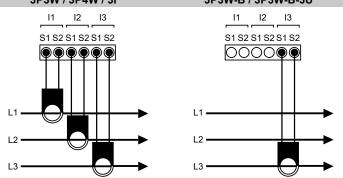
**Note:** Scrupulously respect the matching of phase between the voltage signals and current signals. Failure to comply with this correspondence and connection diagrams gives rise to measurement errors. Do not extend the length of the CT's wires.
