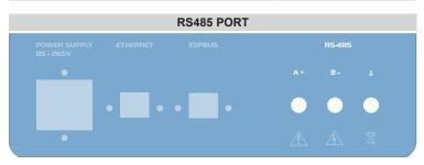
The RS-485 port allows a bidirectional communication in half duplex on a multipoint line and can be used to implement a local communication network.
