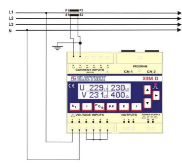
Low Voltage 1 CT (symmetrical and balanced load) Configuration 3Ph/4W-Bal
