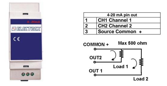
NB. The outputs are self powered; do not use external power supply.
