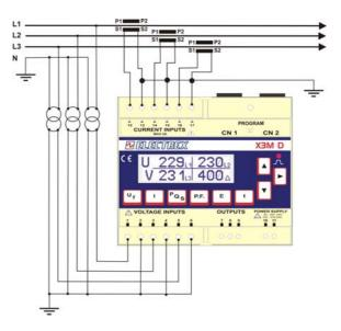
Low voltage 3 CTs Configuration 3Ph/4W High voltage 3 PTs 3 CTs Configuration 3Ph/4W
