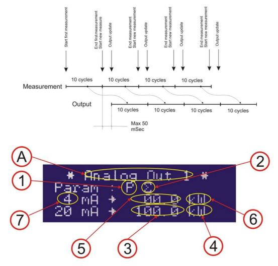
(A) Output identification: **A.o.1** = analog output 1.
