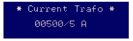
Ensure to enter the CT <u>rated</u> primary and secondary values as indicated on the CT label. When using 2 or 3 current transformers ensure that all the current transformers have the same ratings. The instrument is set by default to **[00005/5]**.
