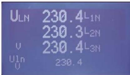
The **Lyra ECT Net H** is equipped with a FSTN dot matrix display with high contrast, back-lighted, white LEDs allowing the simultaneous displaying of 4
