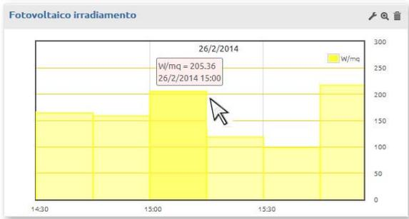
Zoom on the irradiance (w/mq) value measured in a PV system
