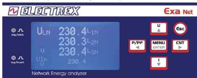
The 6-key keyboard and the display menu column for configuration allow a simple and rational use of the instrument, while the page displayed at start-up can be defined by the user.
